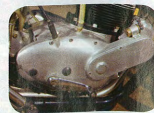
Modified case allows magneto drive from crankshaft
