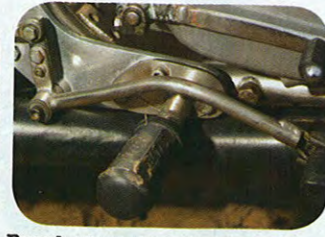
Rear brakes were allowed from '69. Same side as gears though
