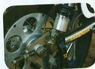
Disc and drive sprocket are interchangeable on the hub
