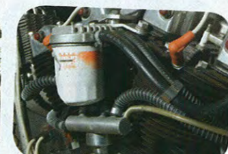
Remote oil filter hides iron barrels and cylinder heads
