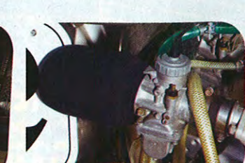
750cc BSA breathes through Mikuni carburetors
