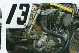
Single carb was used on Sportster derived engine
