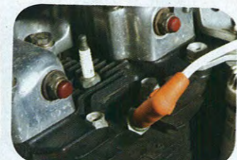
Twin plug heads – but only one is wired for sparks
