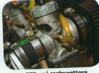
36mm Mikuni carburetors and big air filters
