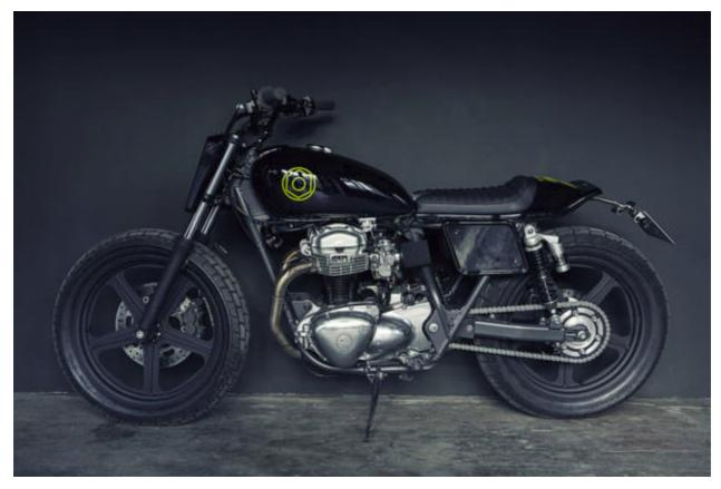
The SuperWheels don't fit the standard Kawasaki fork and swingarm though, so custom-made spacers, caliper brackets and a sprocket carrier are had to be machined up to fit.
